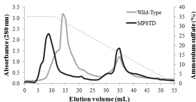
Figure 1. A chromatogram showing HIC purification of the WT and the mutated 8S $\alpha$  globulins. Proteins were eluted at the same retention volume (35 mL) using the decreasing gradient of 35 - 0% ammonium sulphate in 35 mM phosphate buffer 0.4 M NaCl and 1 mM EDTA (pH 7.6).
