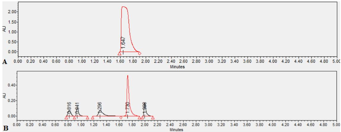
Figure 2. UPLC-based peptide mapping of (A) chemically synthesised LPYPR, and (B) pooled sample of 12- and 24-h tryptic digests of the MP showing the release of LPYPR during the tryptic digestion.
